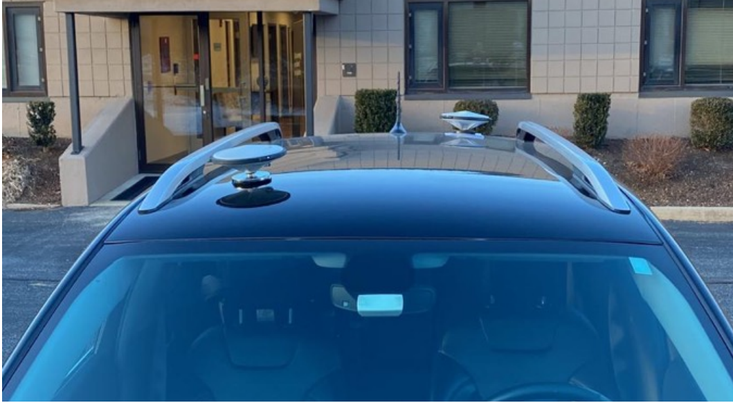
Figure 16: GNSS dual antenna system
