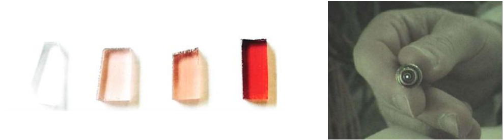
Figure 1: Left, representation of Radiation Induced Attenuation (RIA) with the gradual darkening of a fluorophosphate glass exposed to radiation [2]. Right, Radiation Induced Emission (RIE) resulting in light being emitted and guided by an optical fiber exposed to radiation (courtesy of B. Brichard, SCK-CEN).
