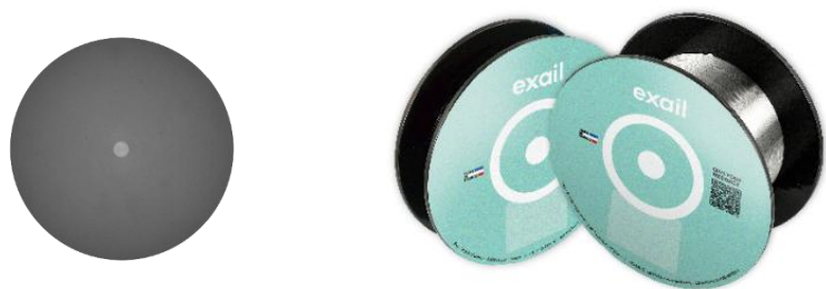
Figure 3 : Left: cleave of a IXF-RAD-SENSE-SM-1550 radio-sensitive fiber designed for RIA dosimetry around 1550 nm.
