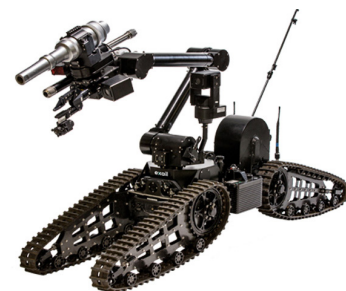
Manipulator arm with CBRN sensor
