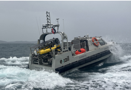
Mine Identification and Disposal Systems (MIDS) configuration.
