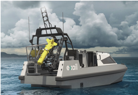
A large aft deck is available to set modular subsystem such as robots or specific sensors.
