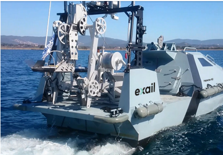
TOWSCA configuration for launching and recovering towed sonars.
