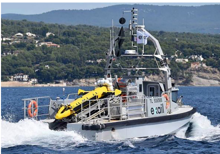
Inspector 125 carrying a mid-size AUV or various towed SAS / SSS with its LARS
