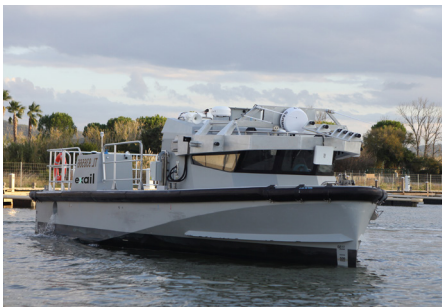
Inspector 125 with a highly reliable multipurpose USV
