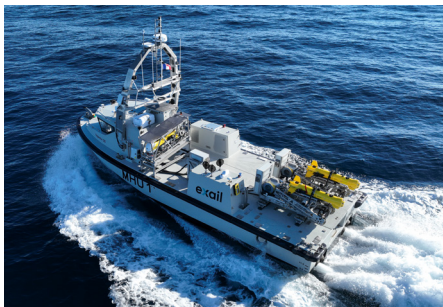
Inspector 125 carrying Seascan-M and K-Ster C for MCM operations
