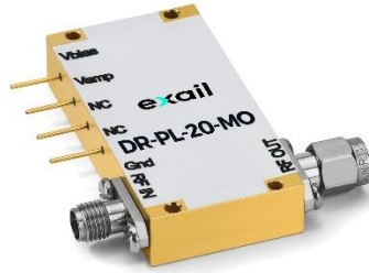
DR-PL-20-MO 20 GHz pulsed modulator driver
