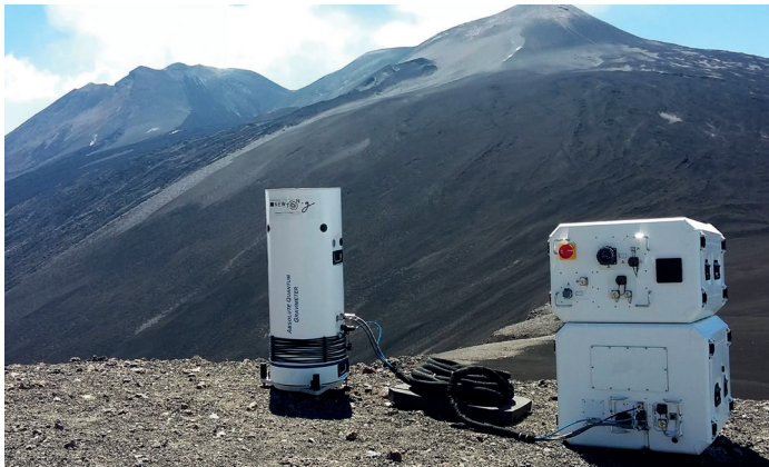
Exail's Absolute Quantum Gravimeter performed the world's first detection of gravity changes induced by volcanic processes (at a level of 10^{-8} m/s 2 )
