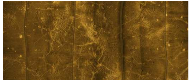
Sams: Mosaic of high-resolution SAS images from multiple survey lines using the Sams sonar
